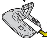
> Remove the battery hatch
