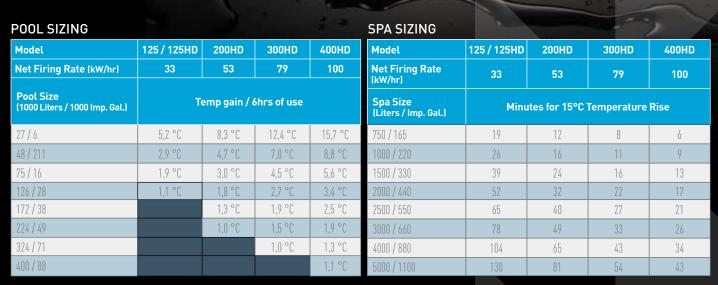
Note: The chart is based on a 15°C temperature rise, discounting losses and only based on heat required to raise temperature in minutes. Two-year limited warranty, See warranty for details.
