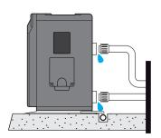
4 - Reconnect and slightly tighten the junctions by hand to prevent the introduction of foreign objects into the HP
