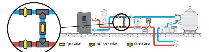
3 - Unscrew the junctions to evacuate all the water contained in the HP.
