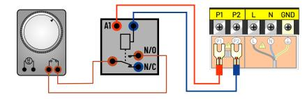
Parameter for taking the connection into account: Check that the setting of the filtration pump parameter (parameter #9) is set to "1". If this is not the case, please contact us to change the setting.
