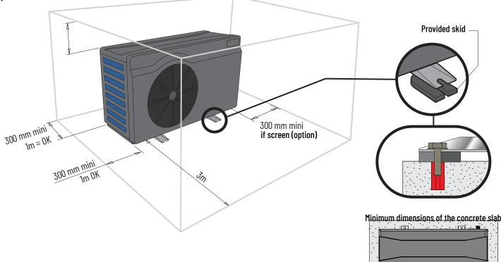
The HP must be installed and maintained on a fixed and solid basis, with the skids placed under the feet.
