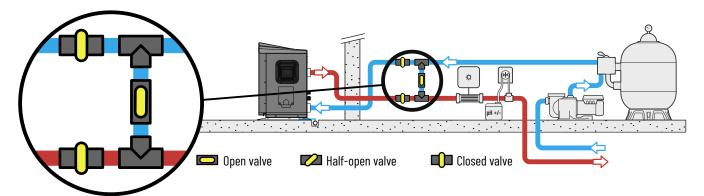
3 - Unscrew the junctions to evacuate all the water contained in the HP.
