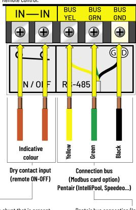
Dry contact input (remote ON-OFF), remove the shunt that is present
