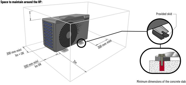
The HP must be installed and maintained on a fixed and solid basis, with the skids placed under the feet.
