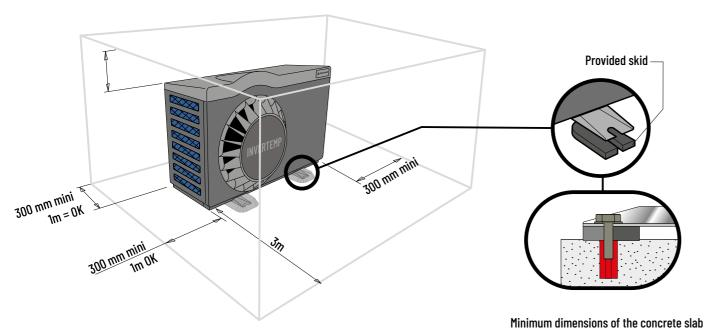
The HP must be installed and maintained on a fixed and solid basis, with the skids placed under the feet.
