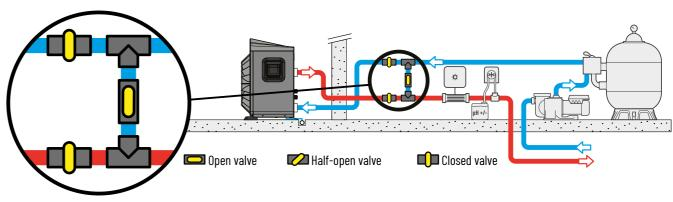
3 - Unscrew the junctions to evacuate all the water contained in the HP.
